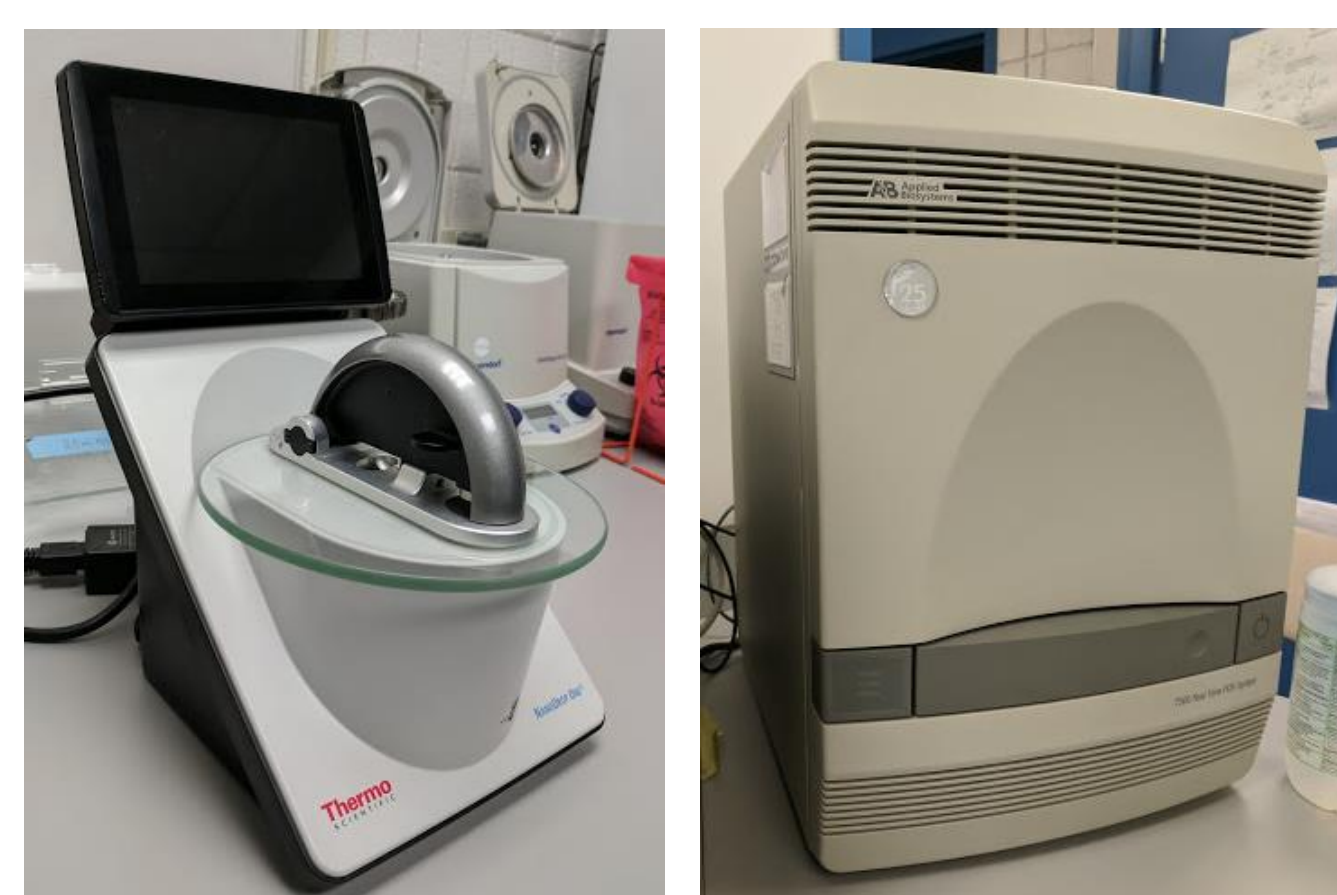
Thermo Scientific NanoDrop One Microvolume UV-Vis Spectrophotometer on left and Applied Biosystems 7500 Sequence Detection System on right.
