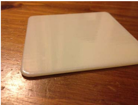
Figure 5 - Flat plate insert after cold acetone bath.
