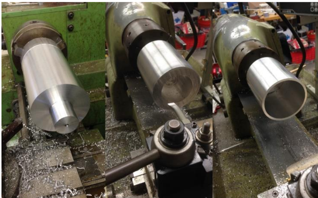
Figure 3. Outer Cylinder construction on lathe
