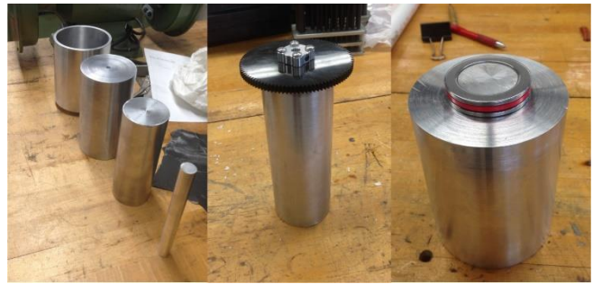
Figure 4. Left: Finished cylinders, Center: gear drive attached to one of the inner cylinders, Right: bearing mounted on outer cylinder
