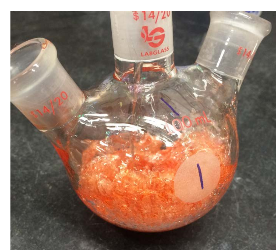
Figure 2. Synthesized poly(4VP- co -AN) with the ratio 100% 4VP to 0% AN.
