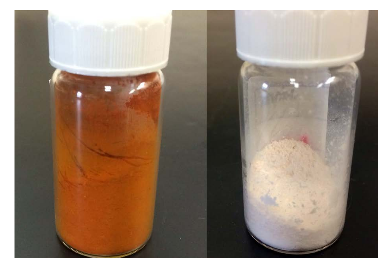
Figure 3. Self-assembly of poly(4VP- co -AN) with Metanil Yellow (left) and Naproxen (right), respectively.
