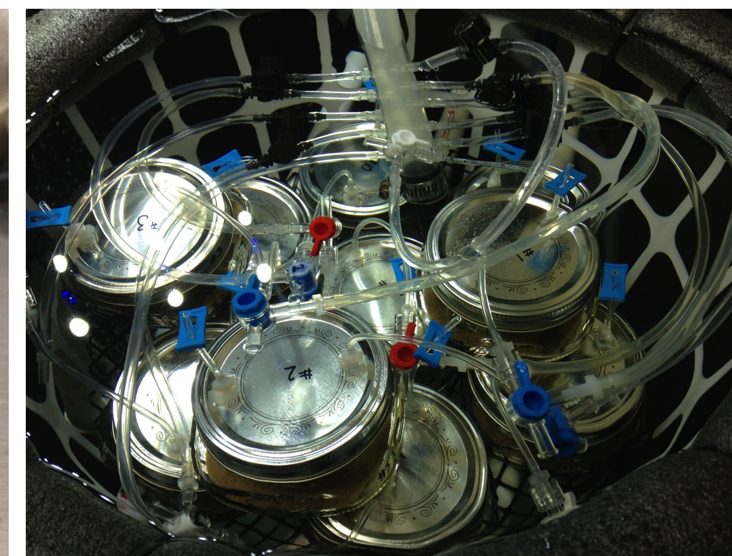
Figure 4: system of ten chambers held below water surface within treatment tank.
