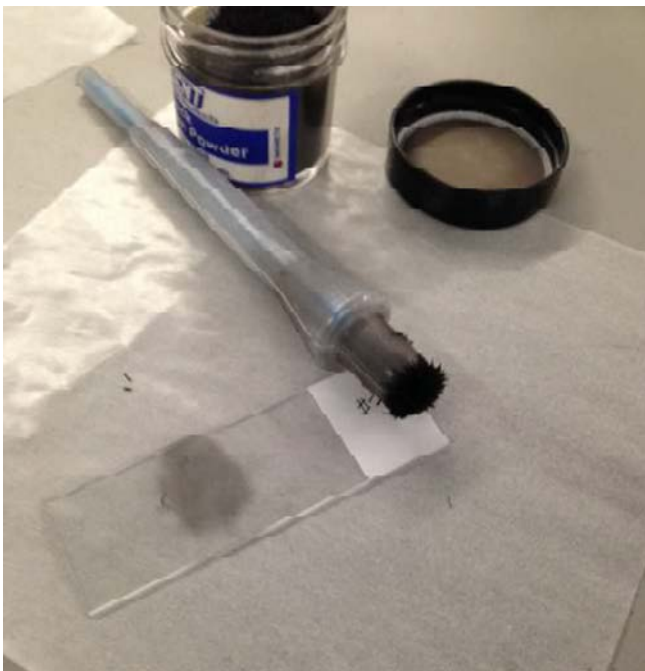
Figure 2: The deposited patent fingerprint residue with the enhancement of magnetic fingerprinting powder.
