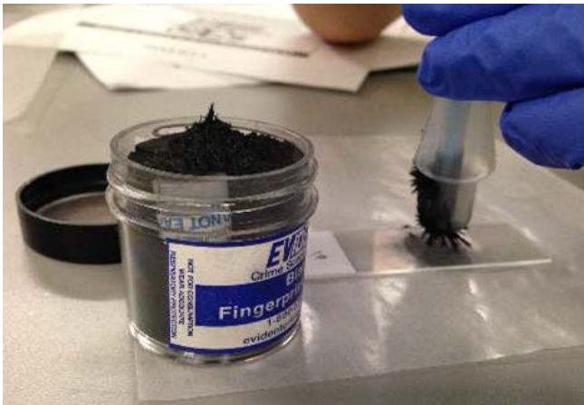
Figure 1: Gently brushing the magnetic powder over the deposited fingerprint residue.
