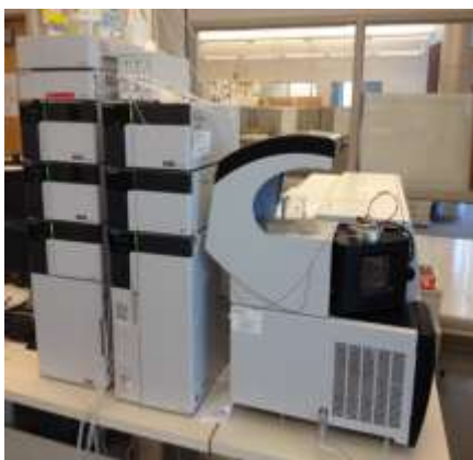
Figure 3: High performance liquid chromatography/triple quadrupole mass spectrometry instrument, located in Connecticut State Crime Laboratory
