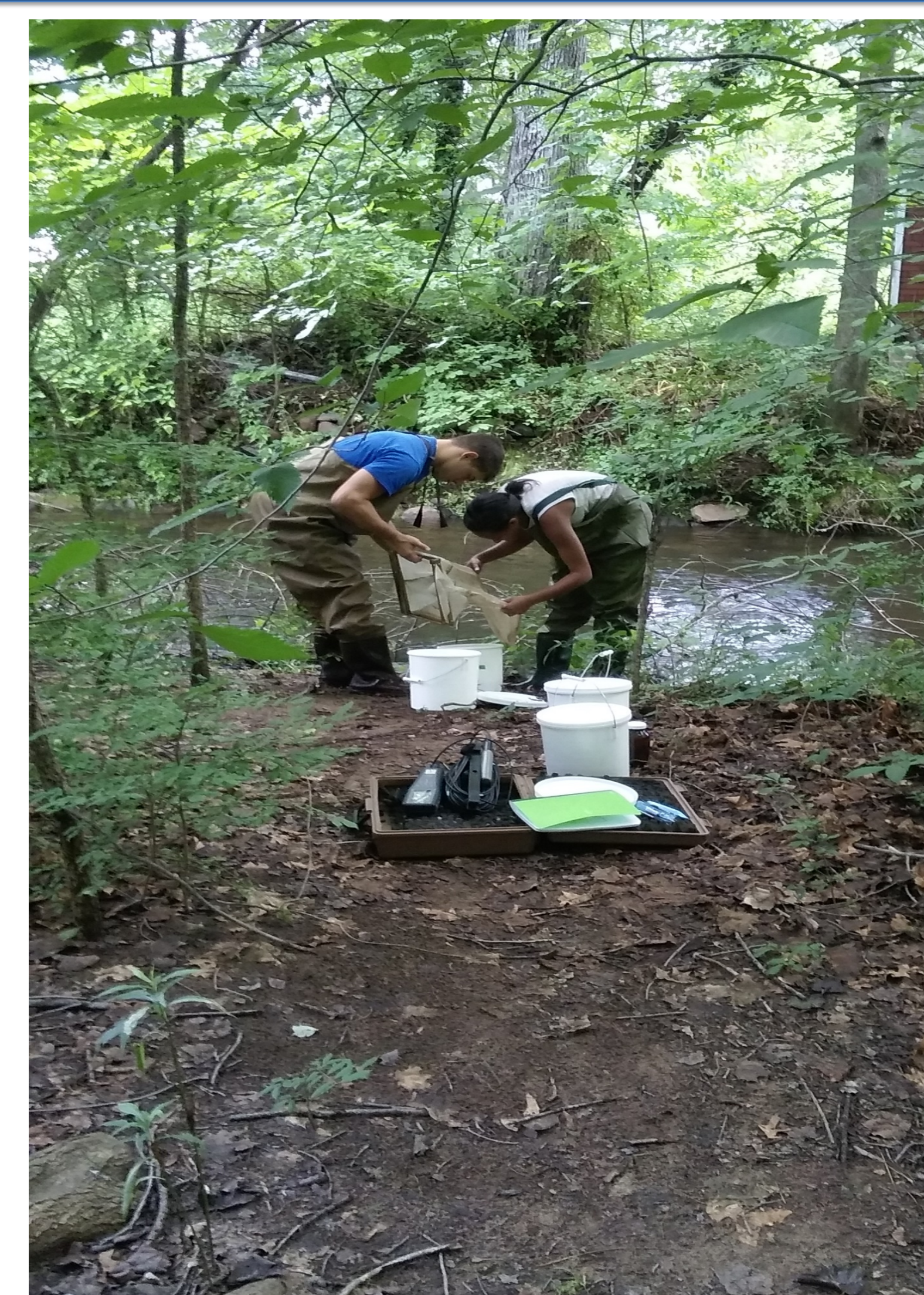
Figure 2. Using the Serber Sampler to collect the macrobenthic community.
